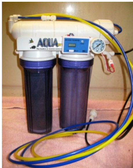
My RO System. The RO membrane is on top, the TDS meter and pressure gage are in front, and the carbon and sediment pre-filters are on the bottom.
